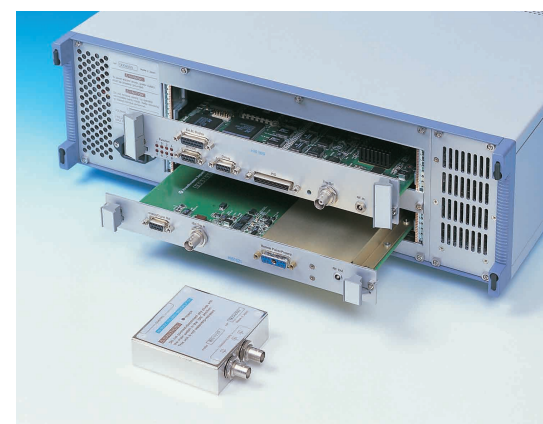
Top : Digital Board Middle : Analog Board Bottom : Remote Pulser/Pre-Amplifier
